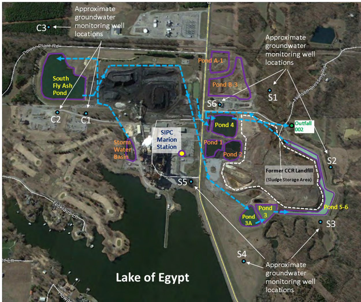
Figure 1: Pond locations and general Site settings. The light blue dashed lines show the water transfer process at the facility through the following sequence: (1) Storm Water Basin, (2) South Fly Ash Pond, (3) Pond 3A/3, (4) Pond S-6, (5) Pond 4, and (6) Outfall 002. Yellow color is used to denote the names of the Ponds included in the petition.
